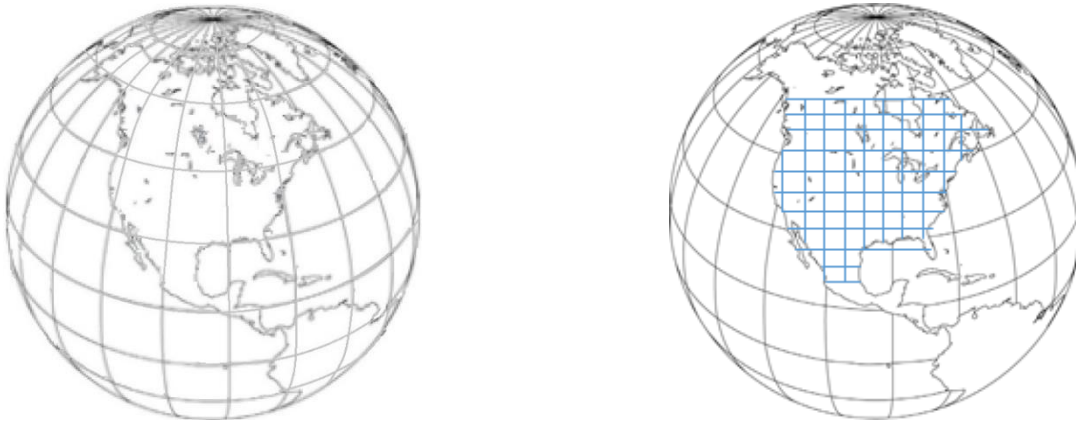
Figure 1: Earth-Centered, Earth-Fixed reference system ( left ) compared to a Plate-Fixed reference system ( right ).
